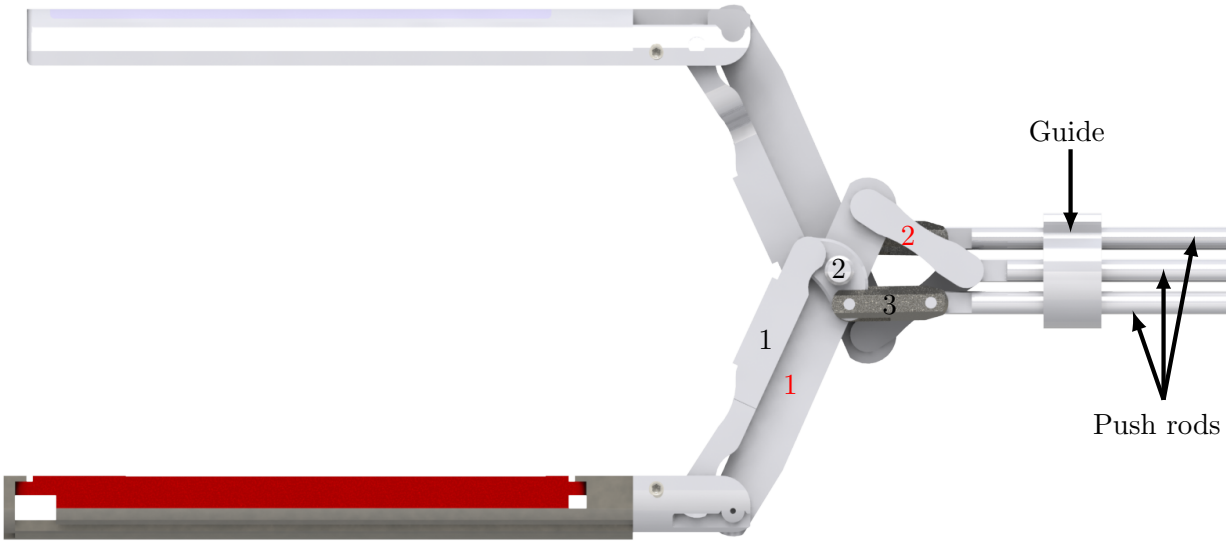
Figure 3.15: Linkage actuation mechanism with push rods. Links of each series are numbered in separate colours.
