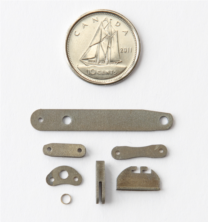
Figure 3.50: Small links machined with wire EDM.
