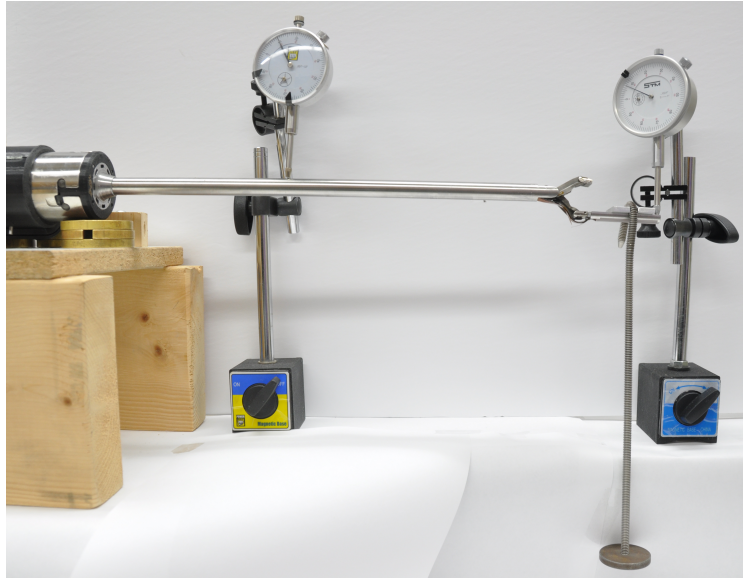
Figure 4.3: Shaft and jaw deflection measurement setup.
