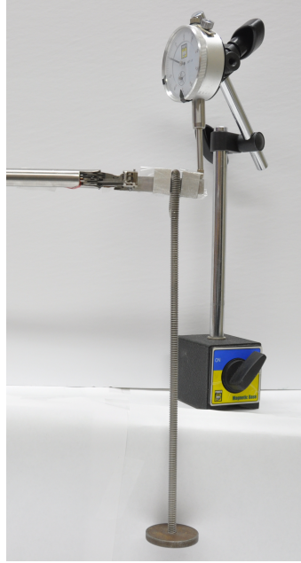
Figure 4.7: Sideways jaw loading setup with an inwards applied load.
